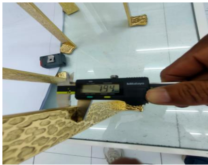
Photo 26) Leg Thickness ( 7.94 mm )
