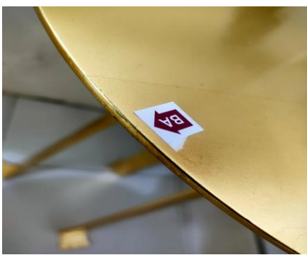
Photo 31) Chipped coating at top edge
